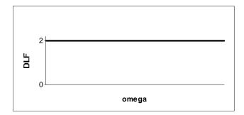
Once the Dynamic Load Factor is known, a static analysis of the system (or of each mode of vibration, when considering multiple degree-of-freedom systems) can be done, with the static results then being multiplied by the DLF to yield the dynamic results. *Note that the DLF is a non-dimensional value that is independent of the applied load*.
