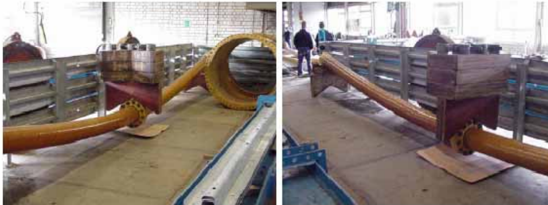
Figure 6; Example; Combined load testing on DN250 PN12.5 Flanged Joint (bending moment & internal pressure, additional moment added by weights)
