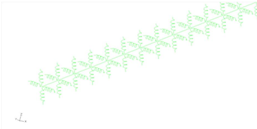
Figure 5: Close-up of a pipeline beam-element model. The springs simulating the soil around the pipeline are discerned. Note that the axial spring is not visible as it was simulated using a vertical oriented spring acting though in the horizontal (axial) direction.
