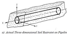
a) Actual Three-dimensional Soil Restraint on Pipeline
