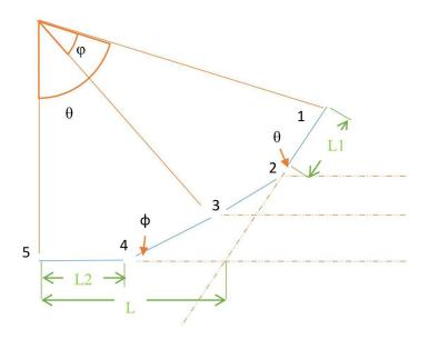
A bend of radius R and of bend angle  $\theta$  is to be split at angle  $\varphi$  for analysis.
