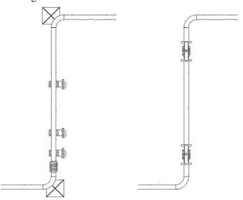
Other piping system types have load bearing hardware in the form of rods, or pinned linkages that restrain the pressure thrust within the expansion joint assembly. These devices, by design, usually limit the bellows movement to just lateral or angular directions.
