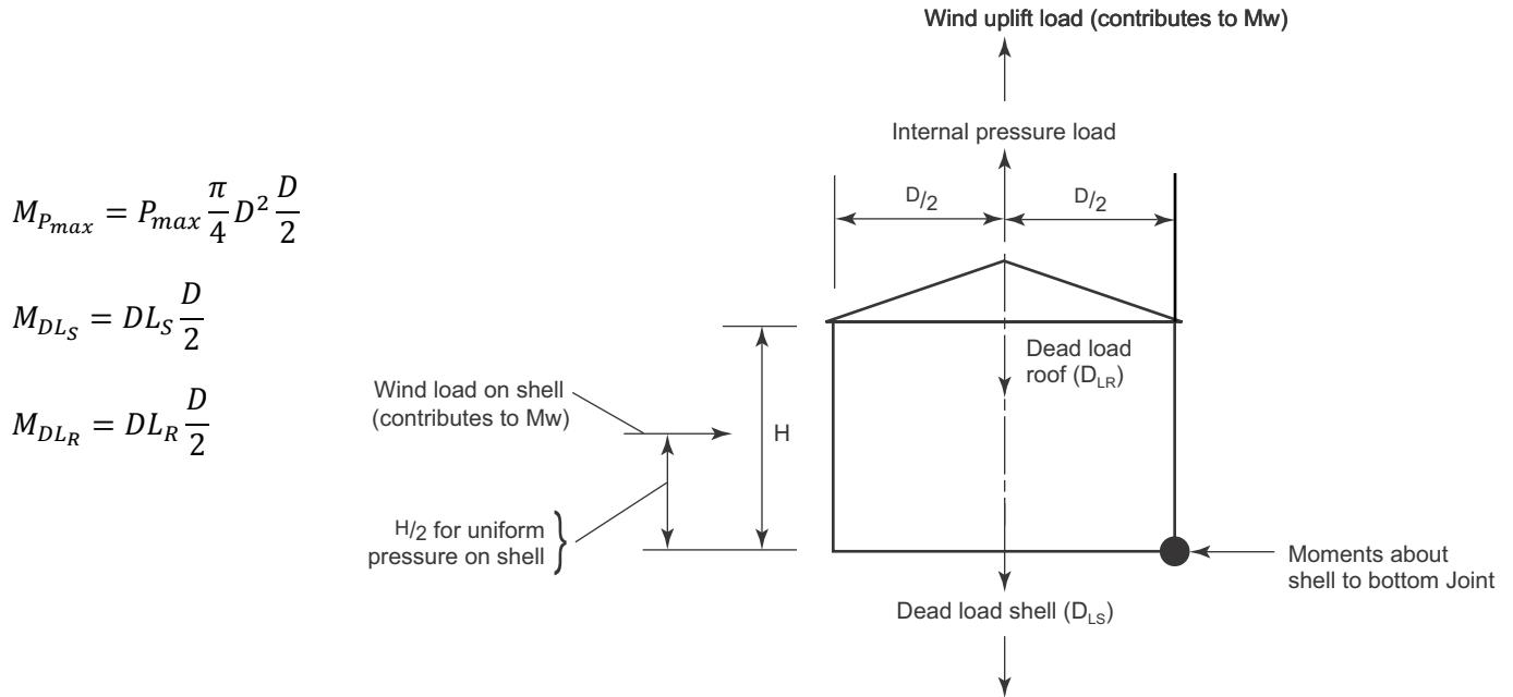
Based on API 650/Figure 5-27—Overturning Check for Unanchored Tanks
